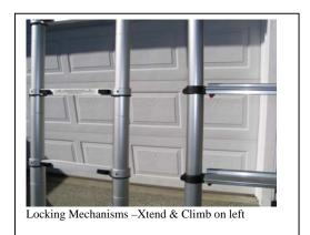
Xtend & Climb® you could raise the top sections. While this won't compromise the integrity of the ladder, it does leave all the sections at the bottom and there is large gap as you step down which could cause a fall. The benefit of this type of locking system is that you can raise or lower just an individual section, so if you misjudge your distances you don't have to lower the ladder all the way.
